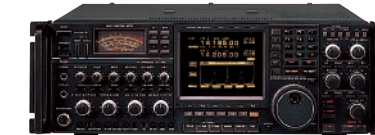
IC-780 (1988) Had a five-inch CRT display and a spectrum scope as standard. Replete with other advanced functions, it became a flagship machine.
