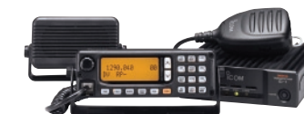
ID-1 (2004) The first D-STAR system compatible digital transceiver opened the future of digital ham radio.
