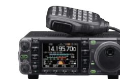
IC-7000 (2005) Compact mobile transceiver covering all HF, 50MHz, 144MHz and 430 (440) MHz bands in one unit. Emergence of the IC-7000 and its IF DSP changes the dimension of the mobile Ham industry.
